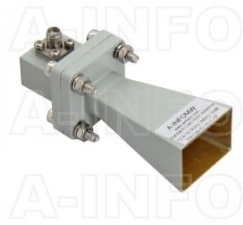
LB-62-10-C-3.5F Standard Gain Horn Antenna 12.4-18GHz 10dB Gain 3.5mm Female
